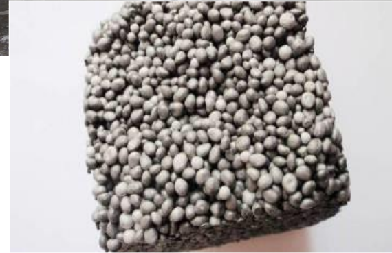
Bonded polystyrene – u-Value 0.7 (50% improvement)
